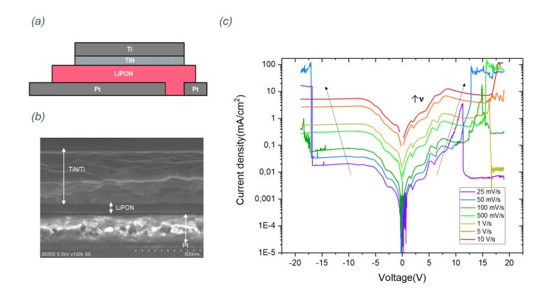
Figure 1 (a) Cross-sectional layout for Pt/LiPON/TiN/Ti microsupercapacitor used for the study, (b) SEM image of LiPON MIM structure, (c) Current density versus voltage for Pt/LiPON/TiN stack of 100nm thick LiPON for scan rates from 25mV/s to 10V/s taken at ambient temperature; the arrows indicate the trend of increase in current density and breakdown voltage with scan rate
