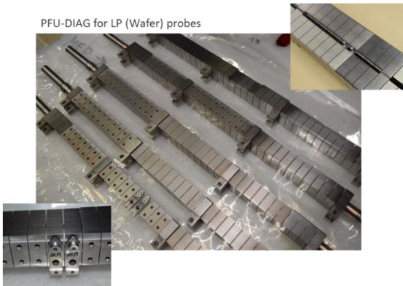
Fig. 11. View of PFUs diagnostic with embedded Langmuir probes (wafer probes)
