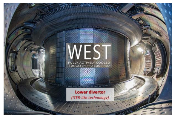
Fig. 1. Overview of the WEST vacuum chamber including the full tungsten actively cooled ITER like divertor
