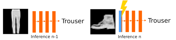
Fig. 7: Illustration of the memory effect when skipping the first convolutional layer.
