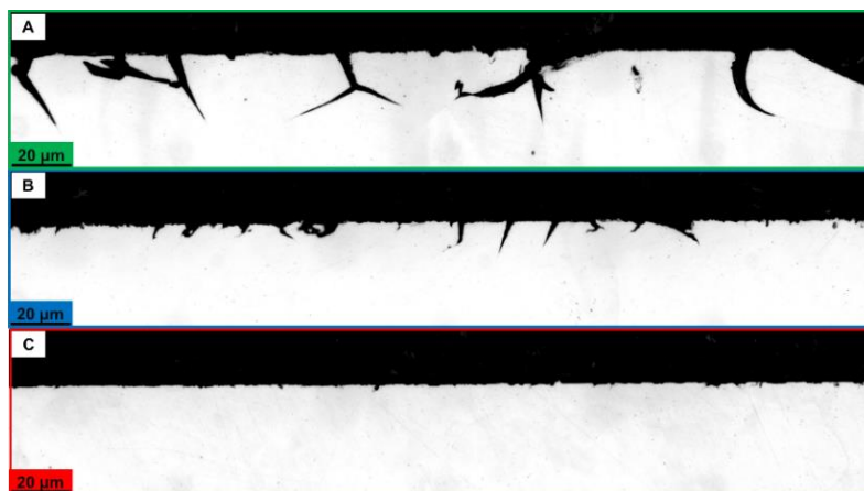
Fig. 7: Cross-sectional observations by optical microscopy after 240 h of immersion in nitric acid containing V(V) at boiling temperature for – (A): Wrought 316L SS, (B): A 316L SS and (C): B 316L SS.
