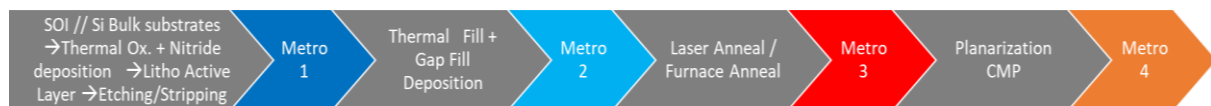
Figure 3: Schematised process flow used in this study, with metrology steps inserted and different technological steps
