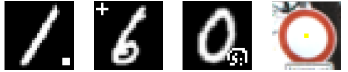
(a) Square pattern attack (b) Cross pattern attack (c) Copyright pattern attack (d) Yellow post-it attack
