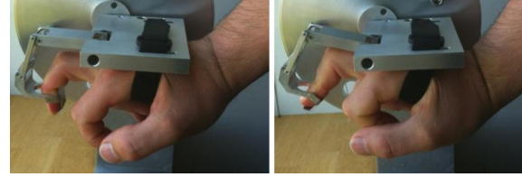
Figure 6: Ability to follow different hand closing trajectories.
