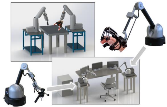
Figure 4: Master slave setup equipped with bi-digital and three fingers grippers.
