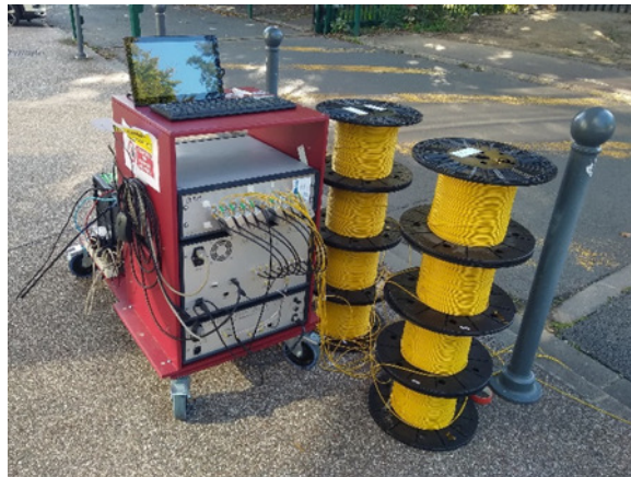
Figure 2.10: MaMIMOSA transmission system with the 500m long RoF links.
