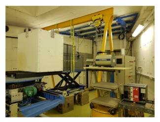
Fig. 12. View of the setup dedicated to the detection of prompt gamma-rays from neutron activation reactions.
