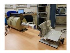
Fig. 3. Photon activation measurement: delayed gamma-ray detection step.
