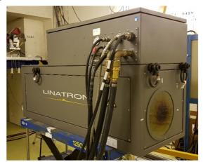
Fig. 1. The Linatron-M9 linac housed at the SAPHIR platform (CEA Saclay, France).
