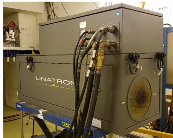
Fig. 1. The Linatron-M9 linac housed at the SAPHIR platform (CEA Saclay, France).
