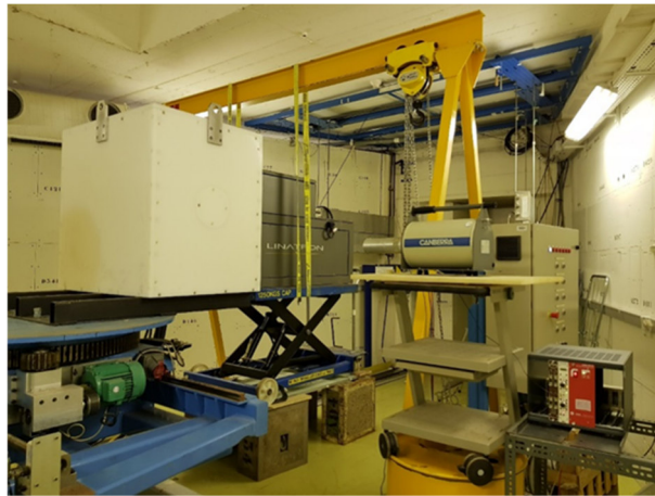
Fig. 12. View of the setup dedicated to the detection of prompt gamma-rays from neutron activation reactions.
