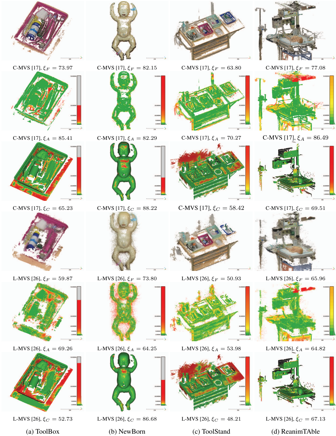
Figure 4: Reconstruction results from the best performing classical and leaned MVS methods [17, 26] across the dataset for \tau = 2mm precision threshold. C-MVS results are shown in top three rows and L-MVS results are shown in the bottom three rows respectively. Rows 1,4 - colored R model; Rows 2,5 - the R model color coded with distance to G visualizes accuracy ; Rows 3,6 - the G model color coded with distance to R visualizes completeness . (Best viewed electronically)
