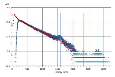
Fig 3. Comparison of the calculated (red) and measured (blue) spectra, configuration 1m, 2 MeV.
