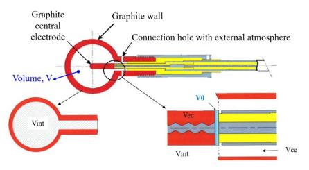
Fig 4. Cut view of the CEA/LNE-LNHB ionisation chamber, red/graphite, yellow/insulator and grey/metal.
