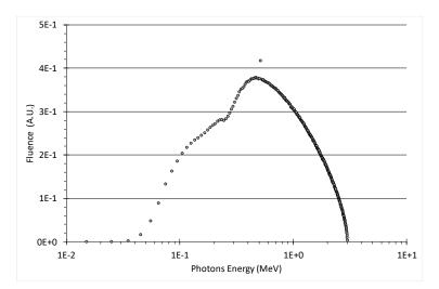
Fig 2. Fluence energy distribution for the configuration 1m, 3 MV calculated with MCNP "tally 5".
