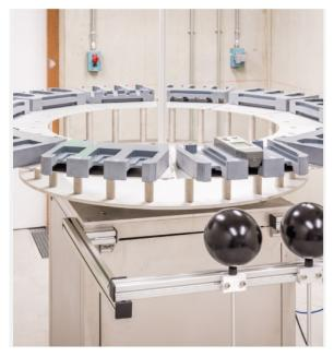
Fig 1. Picture of the sample conveyor with the two monitoring chambers at the front
