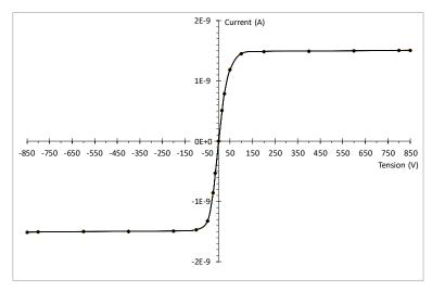
Fig 5. Variation of the current as a function of the high voltage applied to the chamber.
