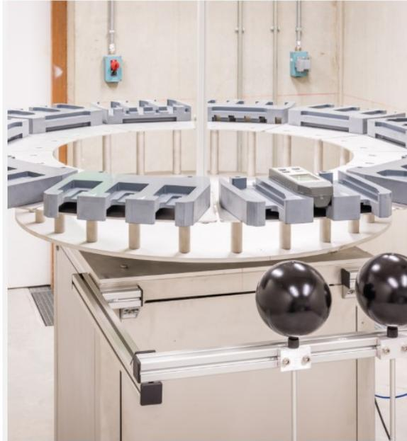
Fig 1. Picture of the sample conveyor with the two monitoring chambers at the front
