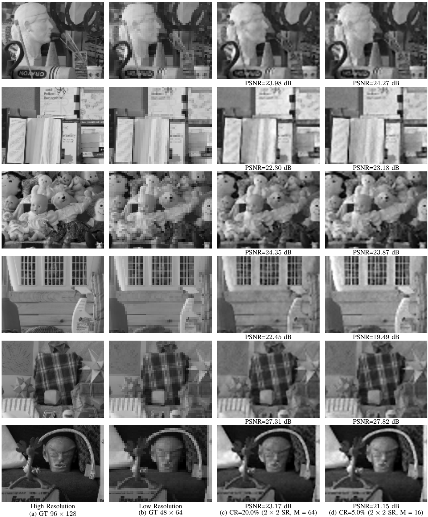
Fig. 12: Intensity SR reconstructions from CS inputs under highly enlightened indoor conditions ( P_a = 350\text{W}/\text{m}^2 ). First and second image columns are respectively groundtruth low resolved and high resolved images for intensity map. While third and fourth ones are 2 \times 2 SR reconstructions issued from the DGM of Fig. 6 at a CR of 20.0% ( 2 \times 2 SR, M = 64 ) and 5.0% ( 2 \times 2 SR, M = 16 ). Note that the reported PSNR are computed from the High Resolution groundtruth images.
