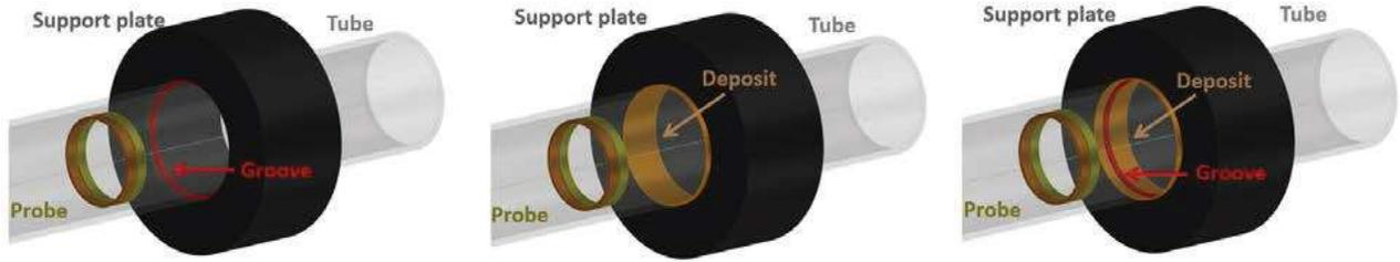
**FIGURE 1.** Configurations of interest: presence of a groove without deposit (left), presence of deposit without groove (center) and presence of both deposit and groove (right).
