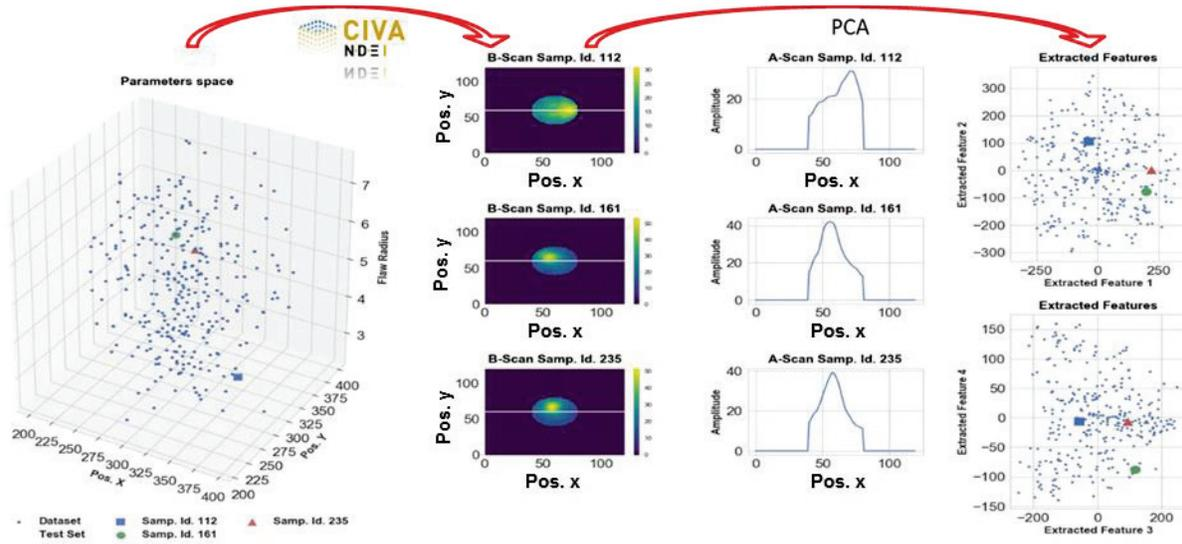
**Figure 4.** From left to right we sketch the set of operation we performed in the training phase targeting classification and regression tasks. On the left, we show the set of parameters generated via LHS design, which have been employed to feed CIVA SHM solver. In the middle, the maps obtained via Excitelet algorithm and the associated projected signals in the PCA space on the right.
