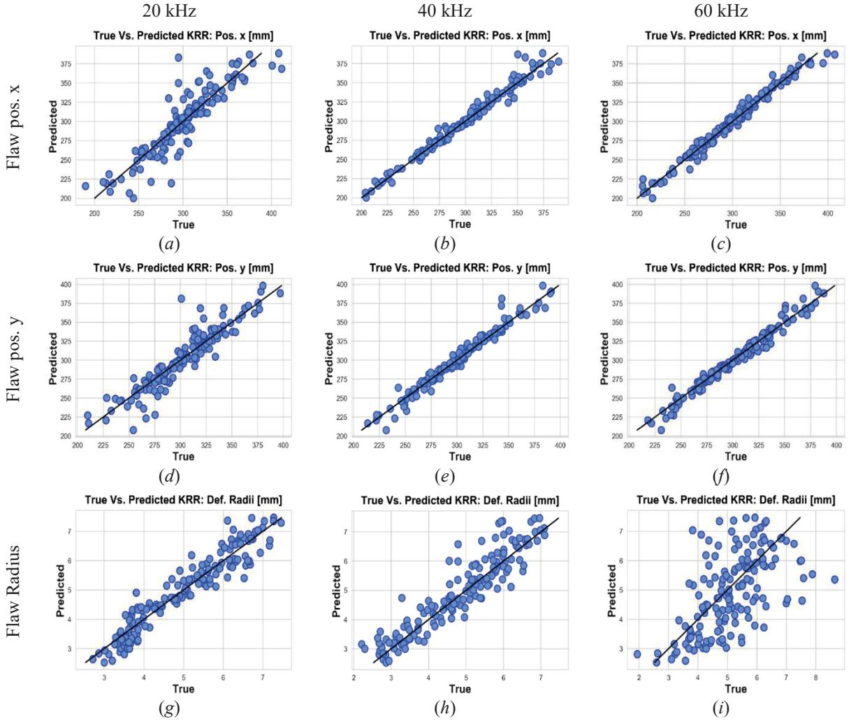
**Figure 6.** KRR predictions are shown via true vs. predicted curves. In (a), (b) and (c) KRR results are provided for flaw position in the x direction and in (d), (e) and (f) prediction associated to flaw positions along y are given at 20 kHz, 40 kHz and 60 kHz, respectively. In (g), (h) and (i) we displayed, in the order, KRR hole radius predictions for the three frequencies considered before.
