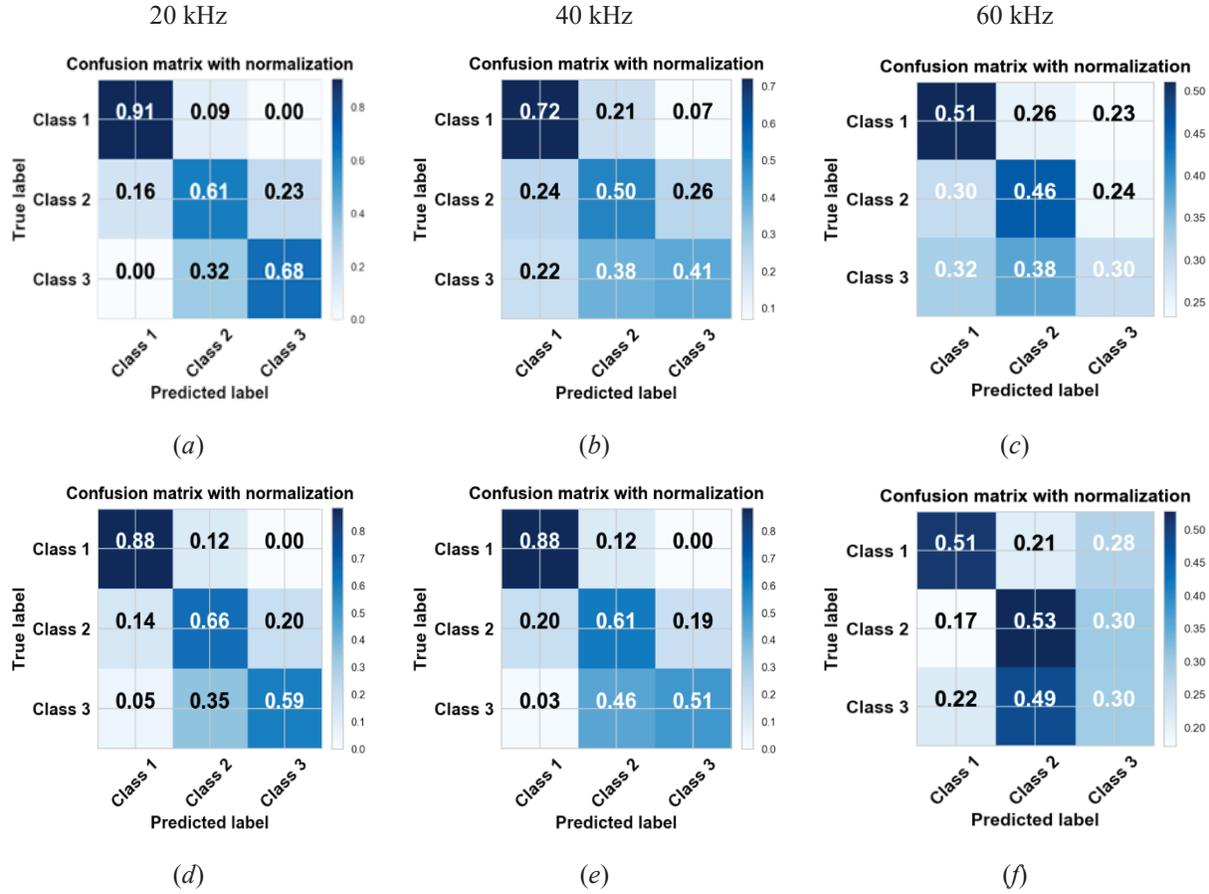
**Figure 5.** Classification results obtained at 20 kHz, 40 kHz and 60 kHz shown through (normalized) confusion matrices. Naïve Bayes classification results are shown in (a), (b) and (c) whereas the SVC results are displayed in (d), (e) and (f).
