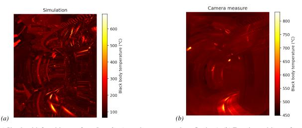
Fig. 2: (*a*) Simulated infrared images from *Speculos* (assuming pure specular reflections). (*b*) Experimental image from WEST wide-angle camera for qualitative comparison with simulation. The parameters used for the simulation do not correspond to the experimental image, hence the different luminosities. For both images, a reflection of the lower divertor pattern can be observed on the upper divertor.
