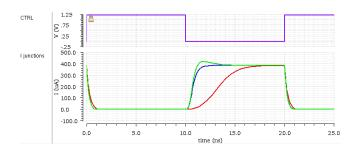
Fig. 4. LEDs junction current whit Ccomp=0 (red), 860fF (blue), 960fF (green).
