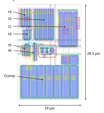
Fig. 6. Pixel circuit layout.
