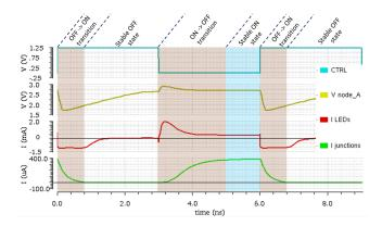
Fig. 5. simulation of the pixel operation.
