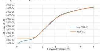
Fig. 1. Characteristic of the static µLED model.
