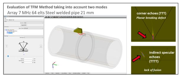
Figure 2 : Simulation of V-Bevel inspection with TFM
