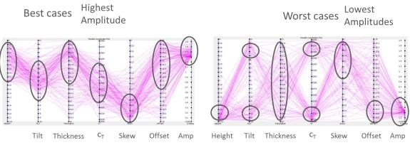
Figure 6: Parallel plot of the parametric evaluation
