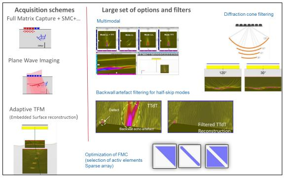
Figure 1: examples of TFM features available on CIVA simulation software
