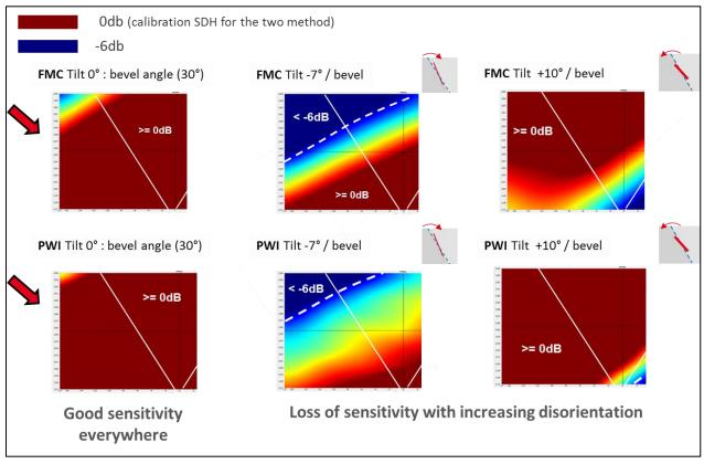
Figure 3: Sensitivity Map for several angles and acquisition schemes
