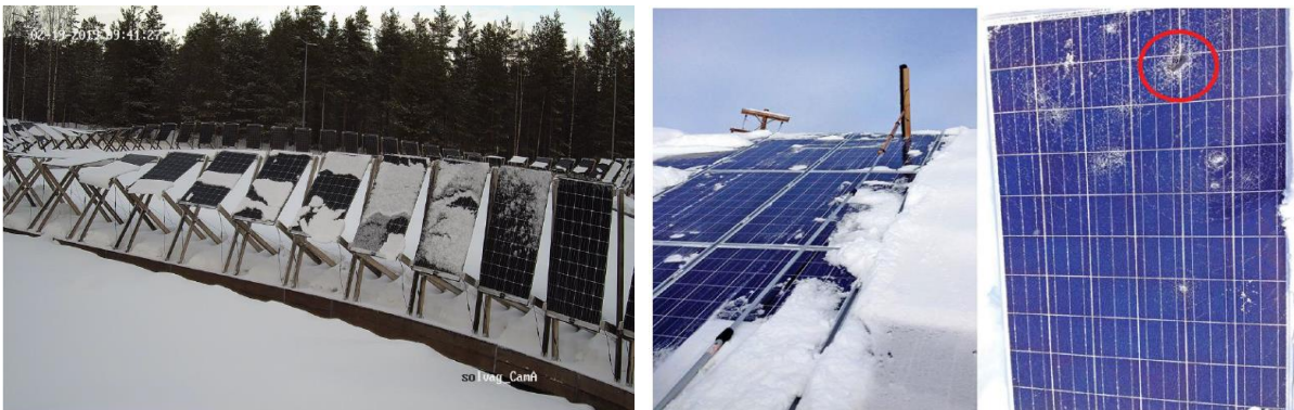
Figure 6: Left: Test site in Piteå, Northern Sweden (65°N) showing the impact of PV array tilt angle on the snow accumulation, for the studied case of frameless bifacial PV modules [6]; Middle and Right: PV module damage due to inappropriate snow cleaning of a PV array [7].
