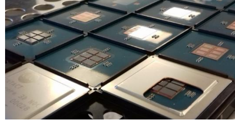
Fig. 5: INTACT integrated circuit [5] with 6 chiplets stacked on an active interposer.
