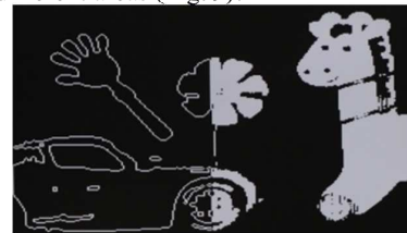
Fig. 9. vision chip in heterogeneous execution mode : edge detection computing on the left, and threshold on the right
