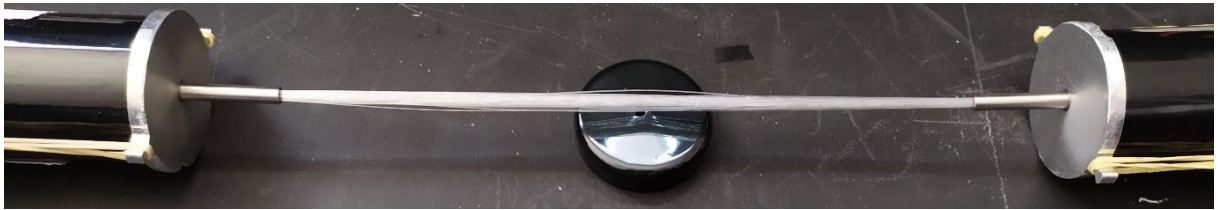
196 Fig. 3. Photography of the experimental setup with scintillating fibres. The bundle of fibres is shown in the middle. The 197 aluminium adaptors to the PMTs are also visible, the mechanical pressure between the fibres and PMTs being exerted by the rubber 198 bands. In the middle is the source holder. Both black cylinders, on the left and right hand sides, are the PMTs.
