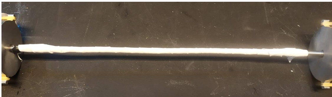
201 Fig. 4. Photography of the experimental setup with scintillating fibres and four PTFE layers stacked (total thickness of 800\ \mu\text{m} ). 202 203
