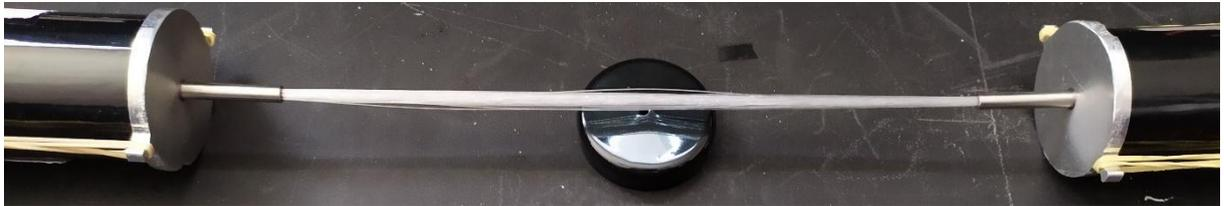
196 Fig. 3. Photography of the experimental setup with scintillating fibres. The bundle of fibres is shown in the middle. The
