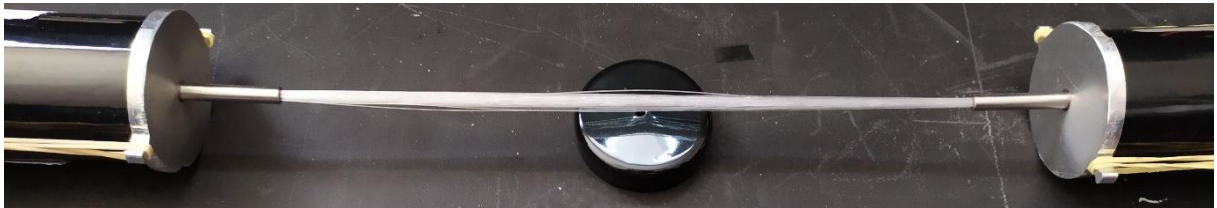
Fig. 3. Photography of the experimental setup with scintillating fibres. The bundle of fibres is shown in the middle. The aluminium adaptors to the PMTs are also visible, the mechanical pressure between the fibres and PMTs being exerted by the rubber bands. In the middle is the source holder. Both black cylinders, on the left and right hand sides, are the PMTs.
