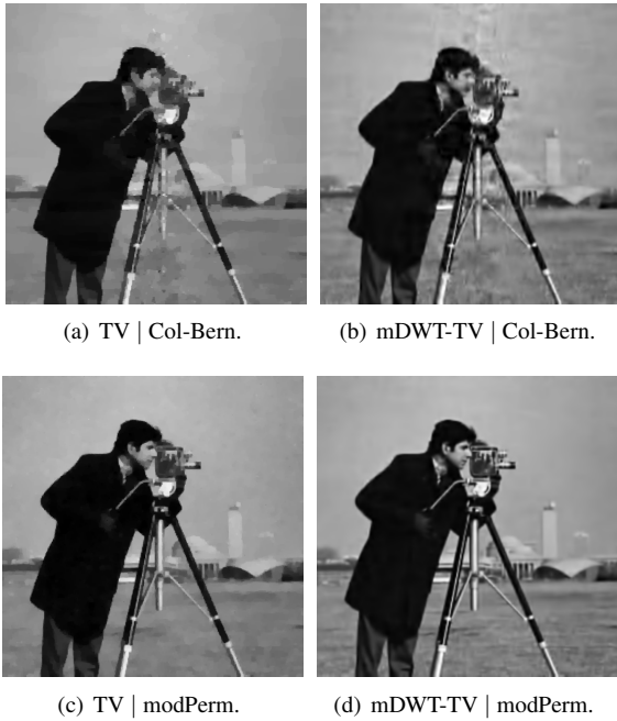
Fig. 4: Quality of reconstruction of our sensing compared to a per-column Bernoulli acquisition scheme (75 snapshots, i.e. , 14.7% compression ratio).
