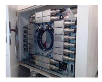
Fig. 6. Integration of C-BORD RRTNIS components in a temperature-controlled and sealed container (in view of further outdoor field tests) at CEA Saclay, France.
