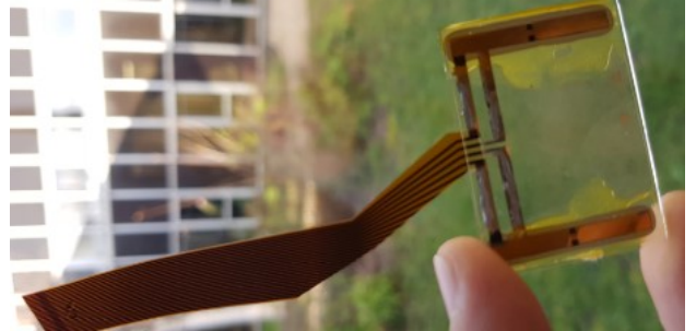
Figure 5: Photography of the 4×3 cm 2 glass plate with the “piezo-in-flex” piezoelectric patch.
