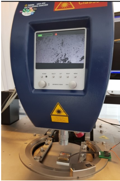
Figure 6: Laser vibrometer POLYTEC MSA400 tool with the haptic plate.
