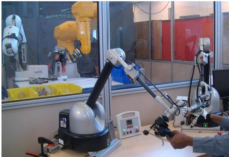
Fig. 16. Master side of the bi-manual dexterous teleoperation platform.
