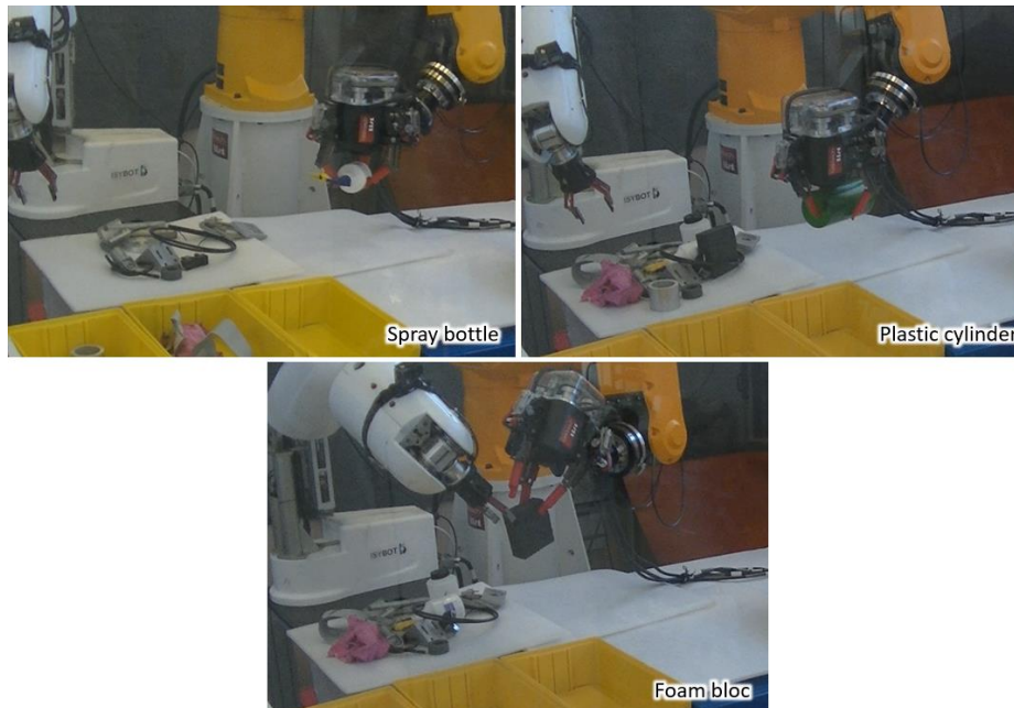
Fig. 21. Grasping various objects in bi-manual teleoperation (adapted from [8]).
