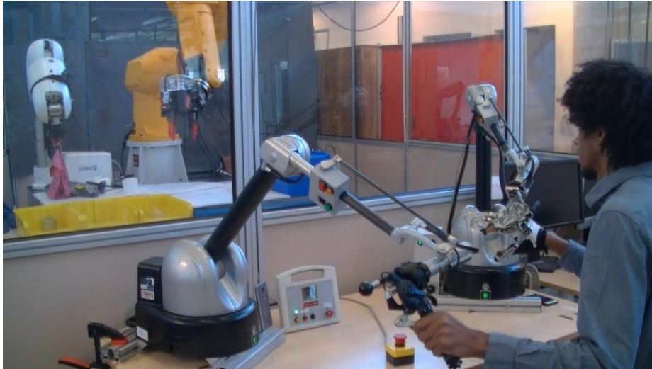
Fig. 1. Bi-manual dexterous teleoperation set-up (source [8]).
