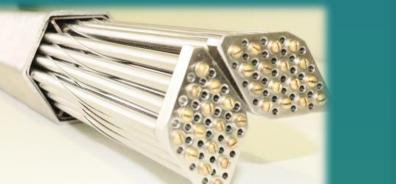
In-pile test device (4696 mm x  $\phi$  219 mm) inserted in the central channel of the **Impulse Graphite Reactor.**
