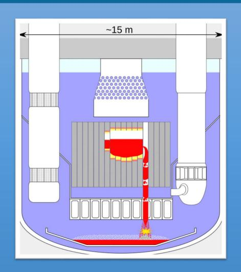
SAIGA Project will provide experimental results of an integral test to validate SIMMER-V calculations on Corium Transfer Tubes
