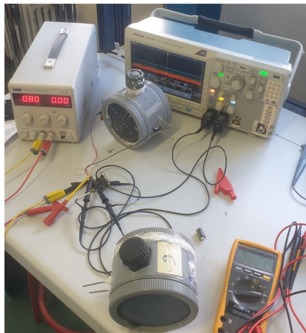
Figure 9. Testbench with the circuit: a lab-scale, batch mode, one-chamber depleted MFC is implemented.
