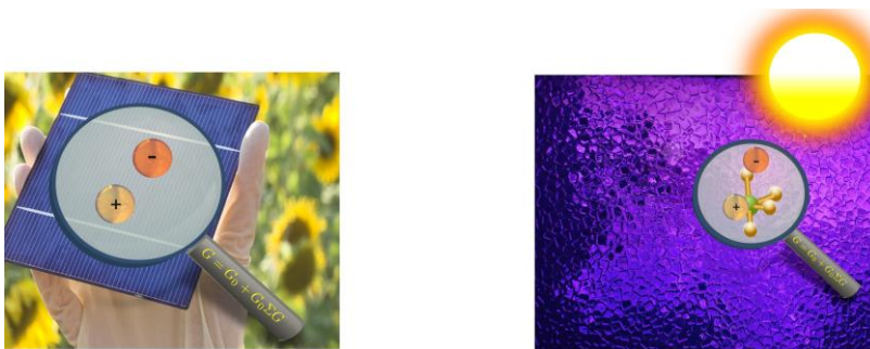
Figure 3.9. Excitons are important in photovoltaics (left illustration) or photocatalysis (right illustration), where electron–hole pairs are created by light absorption and where the transport, separation of charges, and migration of electrons and holes to the desired places is crucial. Theory can help to get insight into these complex processes.
