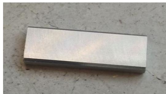
Figure 4: Representative sample of an AVB in Inconel 600.
