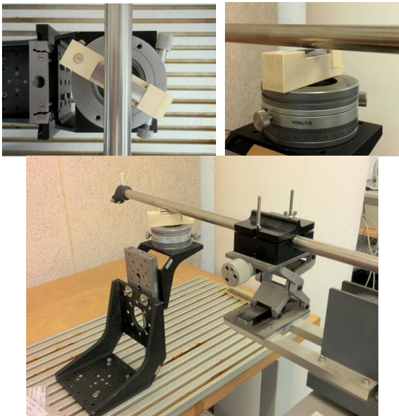
Figure 6: Experimental bench for positioning of the AVB near to the tube inspected.
