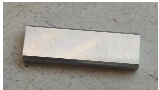
Figure 4: Representative sample of an AVB in Inconel 600.
