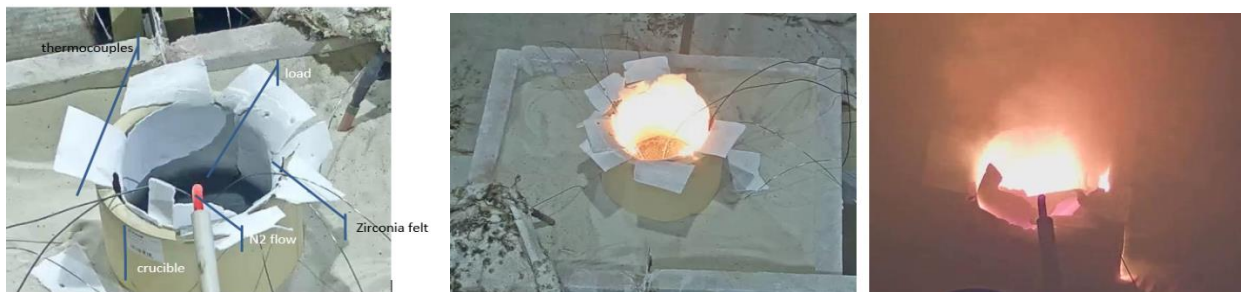
Figure 3: Photographs of test section in VULCANO facility. Left: before heating. Center and Right: during heating phase (Journeau et al., 2022)
