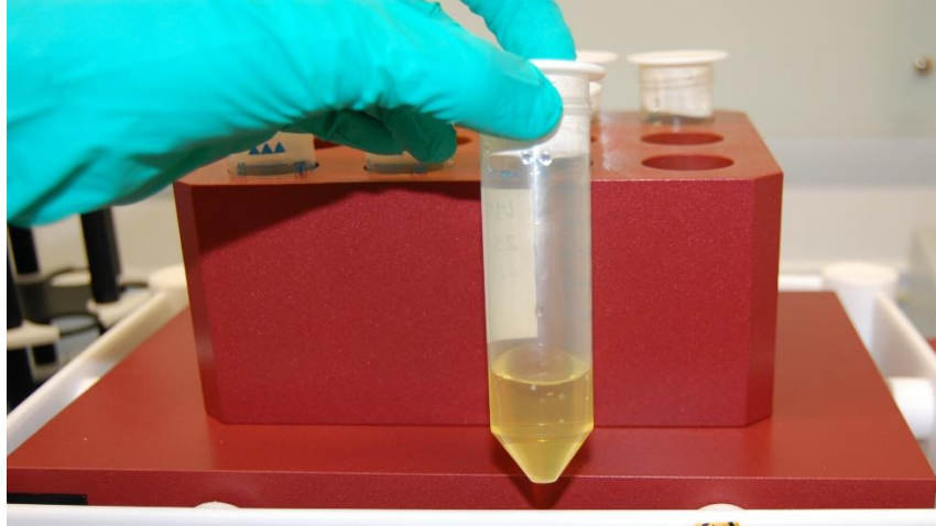
Figure 12: Liquid sample obtained after acidic dissolution over a hot plate. No visible residues.
