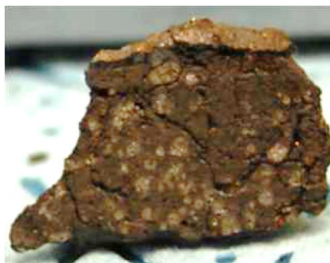
Figure 4: Macrograph of a sample from the fabricated prototypic fuel debris showing zones of different colors (Journeau et al. 2022)
