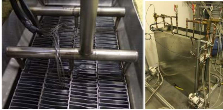
Figure 6: View of the interior of the prototype with the four cavities, the fins and the 5 plate heat exchangers
