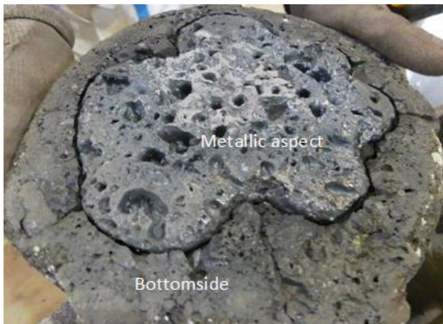
Figure 2 Photograph of simulated fuel debris block obtained by heating and solidification of UO 2 -Ex-Vessel material, taken from the lower side. Oxide and metallic portions were observed.
