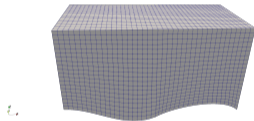
Fig. h Final mesh generated with the 2 Bézier elements defined by the control points of Fig. f
