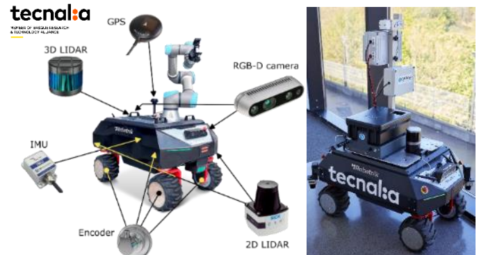
Fig. 9. (Left) RB-VOGUI (Robotnik), and sensors used by Tecnalìa to achieve autonomous navigation and localization of the platform. The platform's dimensions are 104 cm × 65 cm × 56 cm.
