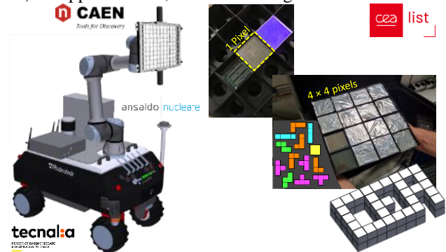
Fig. 8. CAEN's large area α/β PSD phoswich mounted on the robotic arm and CEA List's pixelated plastic scintillator (also to be mounted on the arm).
