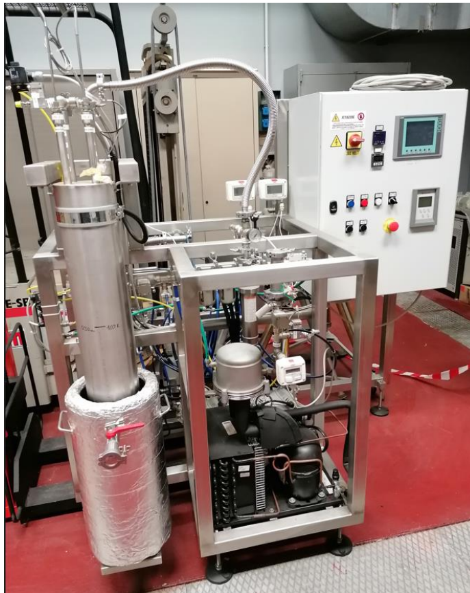
First ENEA-INMRI prototype for gas trapping
