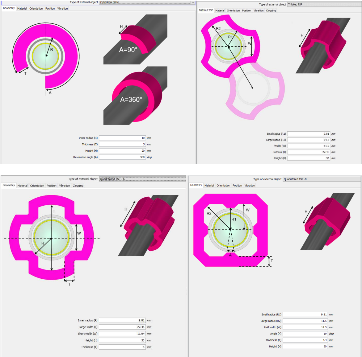
Figure 2. Defining dimensional parameters for tube support plates in the steam generator tube inspection module.
