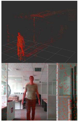
Figure 2: Snapshot of the display of the experimental setup. The top panel shows the filtered PCL representing the data that a real steerable Lidar could provide. The bottom panel shows the filtered PCL superimposed with the image of a webcam for a better understanding of the scene. The difference in the density of points is clearly visible in this representation.
