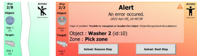
Figure 11. Main information displayed on the HMI (left: nominal mode, right: error alert).
