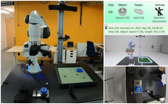
Figure 12. Assembly of the second spacer in autonomous mode. Icons and text are magnified for better readability.
