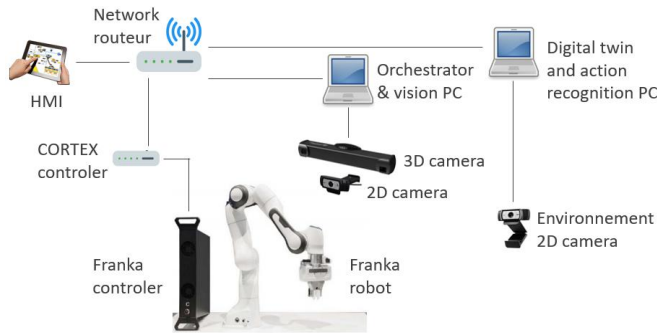
Figure 3. Robot Companion first demonstrator hardware architecture.
