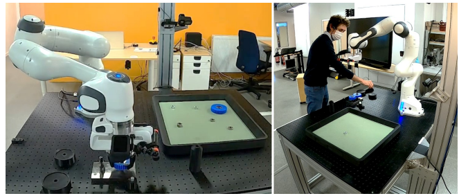
Fig. 4. Insertion of the first gear in autonomous mode (left) and recovery of a failure during the assembly of the second spacer (right).
